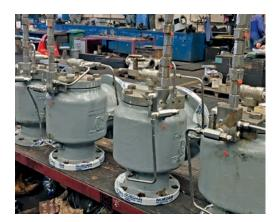
Nordan Marine service team provides service, repair and test of Safety Relief Valves (SRV).
